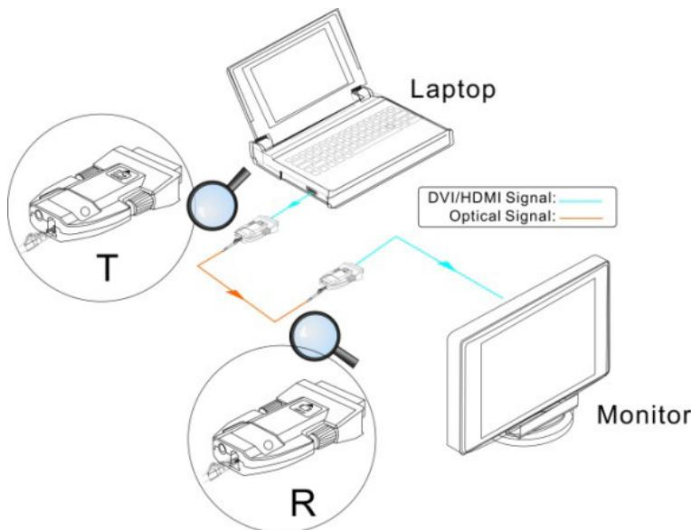
**Step1.** Connect the Transmitter and a DVI source device(e.g.a PC) directly or over a DVI cable.
